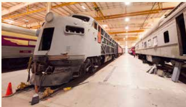
Shop crews have been slowly working on an A-B-A set of F units for use on special trains. At right is a former Southern Pacific office car under restoration. Two photos, TRAINS: Jim Wrinn
